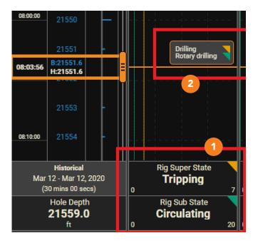
If you're using Pason Live, the real-time 1 and reading bar 2 values are automatically displayed in text form, so you can easily see the activity with the need to reference this table.
