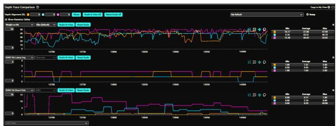
Use **Depth Trace Comparison** to view vibration information and compare drilling parameters across multiple wells.
